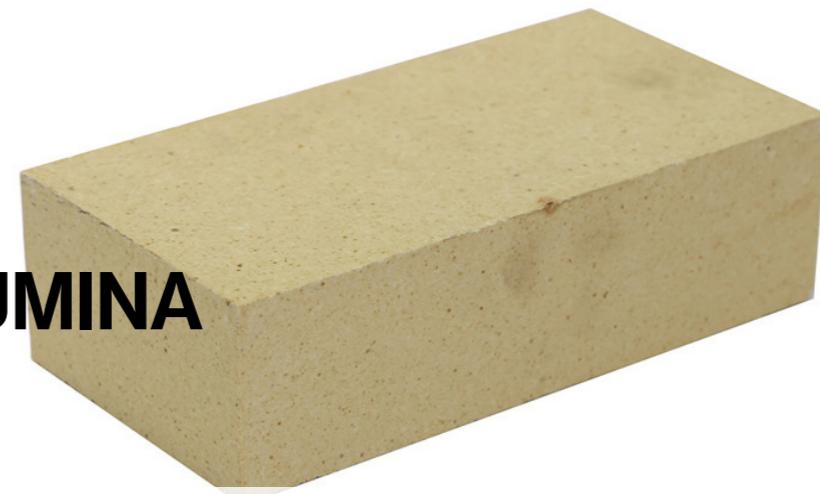
High alumina bricks of over SK35 contain over 45% Alumina and are made from raw materials of unusually high degree of purity of Bauxite and refractory clay. For serve under severe conditions, JUCOS Alumina bricks have excellent mechanical strength, good resistance to thermal spalling, and are highly resistant to chemical attack by volatile alkalis and some slag. We manufacture and design alumina bricks to meet the requirements of a great variety of service conditions thorough quality control.
